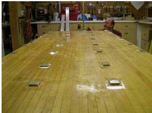
The melamine would serve as an assembly surface for the torsion box, as well as be the bottom half of a vacuum box, which would be used to clamp the torsion box while the glue cured. (more details later)
