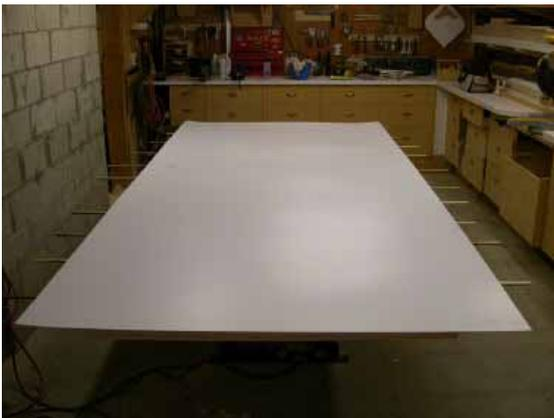
With the lip installed flush to the surface of the box, I was ready to skin the surface of the bench with white plastic laminate. Laminate would provide a surface that is durable, easy to clean, and can also be used for full size sketches or drawings, if necessary. 3M waterbase contact cement was used to attach the laminate skin. Once the laminate was trimmed to size, a small chamfer was routed into the edge of the bench to help protect it from dings.
