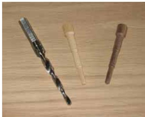
All you need to use the dowels are a Miller TruFit drill bit, which is a stepped bit similar to the Kreg pocket hole bit, and of course, Miller Dowels. The bits and dowels are sold together as a kit or can be purchased separately. There are three sizes available; 1X for pieces up to 1 1/8" thick, 2X for pieces up
