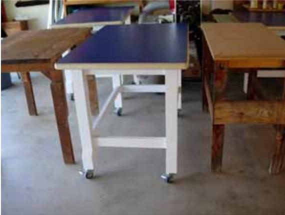
The 4x4 legs were not big enough to seat the mounting plates for my casters, so I added a piece of 6/4 redwood to the base of the legs. To keep the costs down I used construction grade common for the legs (it's normally used for fence posts) and kiln-dried studs for the stretchers and aprons, all of which I ran through my planer for a consistent thickness.
